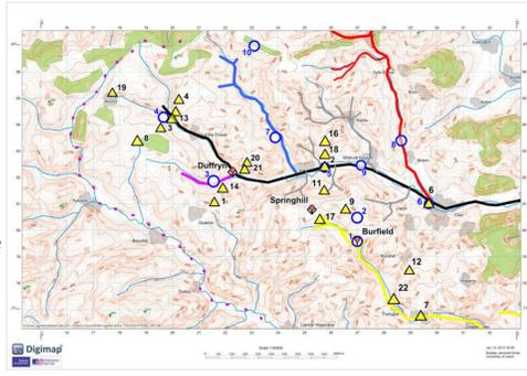
Above: Map showing instrumentation deployed during COLPEX, situated across the Clun valley region. Triangles are HOBOS, circles are AWS, balloons are flux tower sites.
