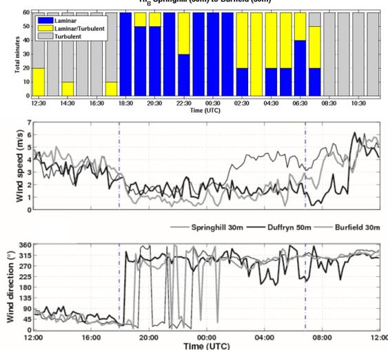
Fig.5. Top, bulk Richardson number ( $Ri_B$ ) representing region between the hill top (Springhill, 30m AGL) and Burfield valley (Burfield 30m AGL). Bottom. Time-series of wind speed and direction for three mast sites.
