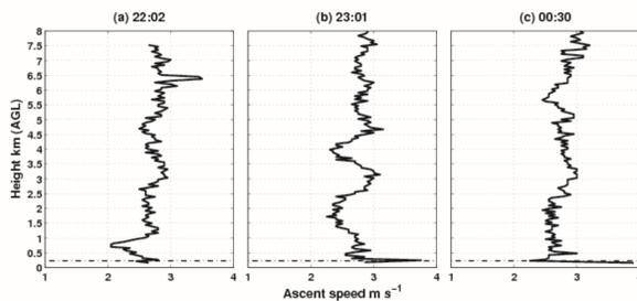
Fig.4. Radiosonde ascent speed profiles launched from the valley floor site Duffryn.
