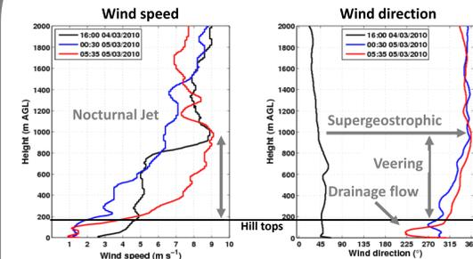
Fig.6. Radiosonde profiles launched from valley floor site Duffryn, showing wind speed and direction with height above ground level.
