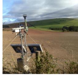
Pictured right: AWS 2, one of 10 University of Leeds and NCAS Automatic Weather Stations (AWS) deployed during COLPEX.
